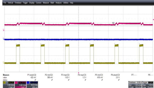
Figure 39 – Output Voltage and Current Waveforms. 265 VAC Input. Upper: 5 V, 1 V, / div. Middle: 55 V, 10 V / div. Lower: I_{OUT} , 1 A , 1 s / div
