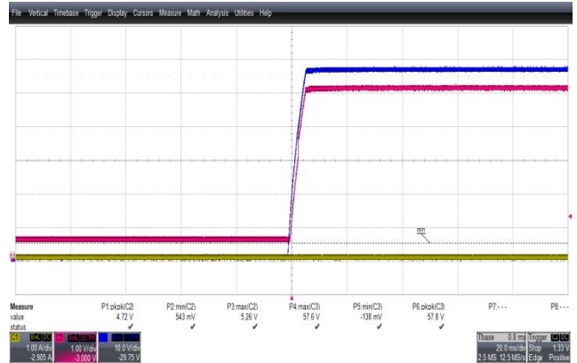
Figure 37 – Output Voltage and Current Waveforms. 265 VAC Input. Upper: 5 V, 2 V / div. Middle: 55 V, 10 V / div. Lower: I OUT , 1 A, 20 ms / div.
