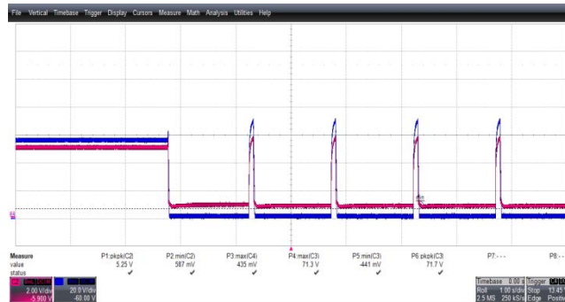
Figure 40 – Output Voltage Waveform. 90 VAC Input. Upper: 55 V, 20 V / div. Lower: 5 V, 2 V / 1 s / div.
