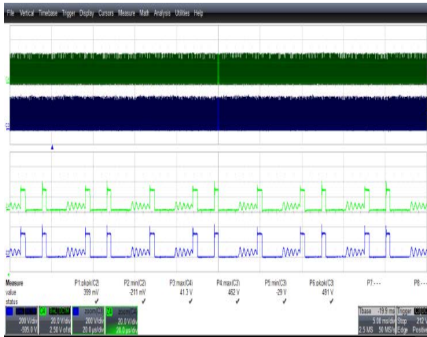
Figure 32 – SR FET and Output Diode Voltage Waveforms. 265 VAC Input, Full Load. (462 V MAX for 55 V, 41.3 V MAX for 5 V.) Upper: 5 V, 20 V /, 5 ms, 20 μs / div. Lower: 55 V, 200 V / div.
