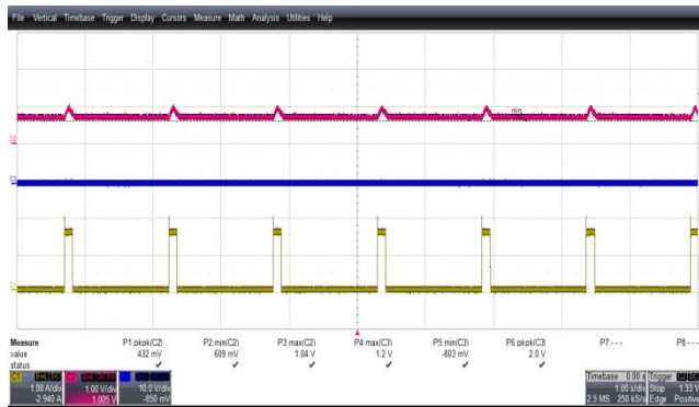
Figure 38 – Output Voltage and Current Waveforms. 90 VAC Input. Upper: 5 V, 1 V, / div. Middle: 55 V, 10 V / div. Lower: I_{OUT} , 1 A , 1 s / div.
