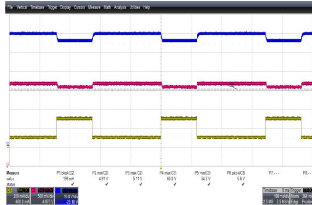
Figure 27 – 0.1 A – 0.32 A, 55 V Load Step Transient Response. 265 VAC. 5 V_{MIN} : 4.91 V. 5 V_{MAX} : 5.11 V. 55 V_{MIN} : 54.3 V. 55 V_{MAX} : 60 V. Upper: 55 V OUT , 10 V / div. Middle: 5 V OUT , 0.5 V / div. Lower: 55 V Load, 0.2 A, 100 ms / div.
