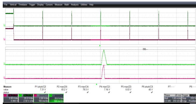
Figure 41 – Output Voltage Waveform. 265 VAC Input. Upper: 55 V, 20 V / div. Lower: 5 V, 2 V / 1 s / div.
