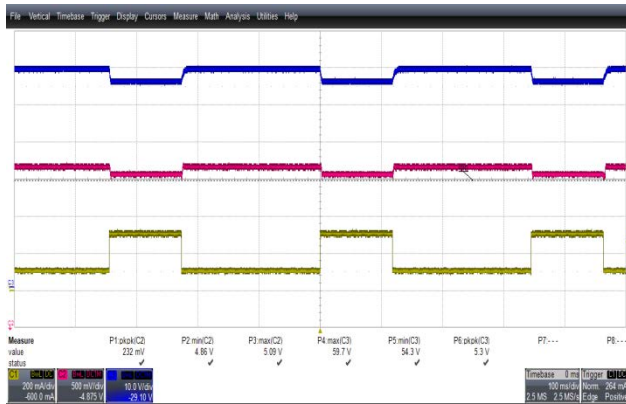
Figure 26 – 0.1 A – 0.32 A, 55 V Load Step Transient Response, 90 VAC. 5 V_{MIN} : 4.86 V. 5 V_{MAX} : 5.09 V. 55 V_{MIN} : 54.3 V. 55 V_{MAX} : 59.7 V. Upper: 55 V OUT , 10 V / div. Middle: 5 V OUT , 0.5 V / div. Lower: 55 V Load, 0.2 A, 100 ms / div.
