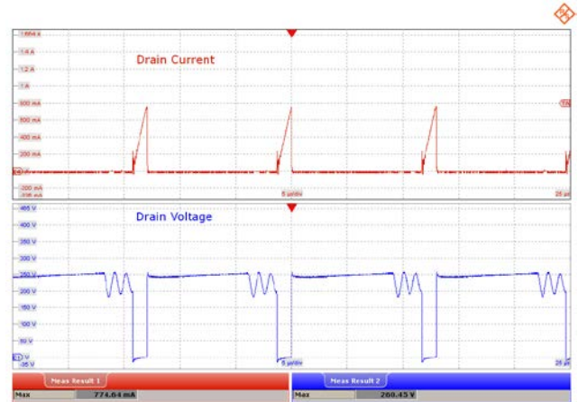
Figure 42 – 185 VAC, 30 V LED Load. Upper: I_{DRAIN} , 200 mA / div. Lower: V_{DRAIN} , 50 V / div., 5 \mu s / div. Peak I_{DRAIN} : 774.64 mA. Peak V_{DRAIN} : 260.45 V.
