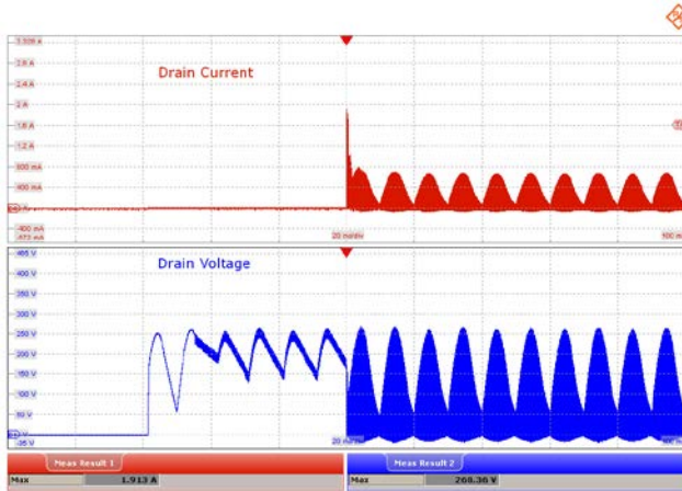
Figure 47 – 185 VAC, 30 V LED Load, Start-up. Upper: I_{DRAIN} , 400 mA / div. Lower: V_{DRAIN} , 50 V / div., 20 ms / div. Peak I_{DRAIN} : 1.913 A. Peak V_{DRAIN} : 268.36 V.
