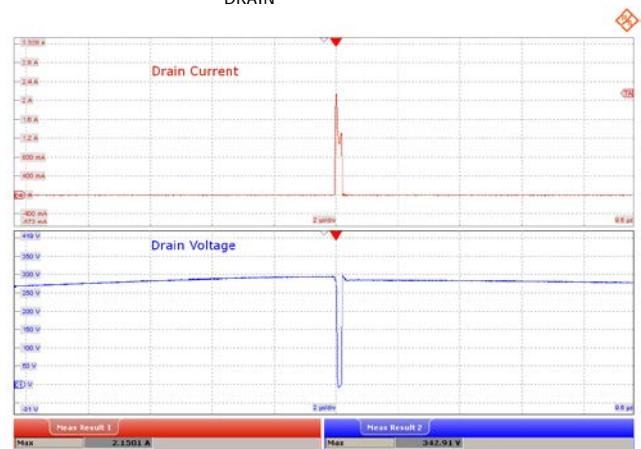
Figure 54 – 185 VAC, Output Short. Upper: I_{DRAIN} , 400 mA / div. Lower: V_{DRAIN} , 50 V / div., 2 µs / div. Peak I_{DRAIN} : 2.1343 A. Peak V_{DRAIN} : 275.72 V.
