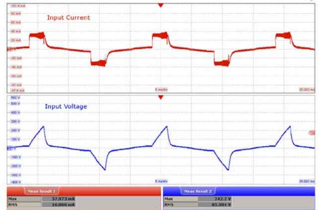
Figure 82 – 52° Conduction Angle. Upper: I_{IN} , 20 mA / div. Lower: V_{IN} , 100 V / div., 5 ms / div. Peak V_{IN} : 242.2V. V_{RMS} : 85.304 V
