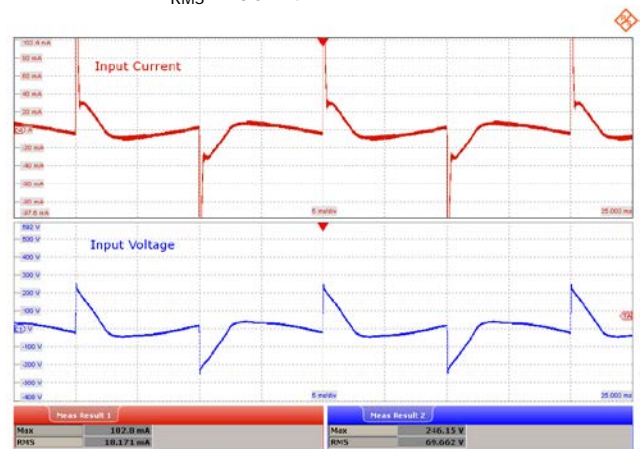
Figure 72 – 120° Conduction Angle. Upper: I_{IN} , 20 mA / div. Lower: V_{IN} , 100 V / div., 5 ms / div. Peak V_{IN} : 325.2 V. V_{RMS} : 206.24 V
