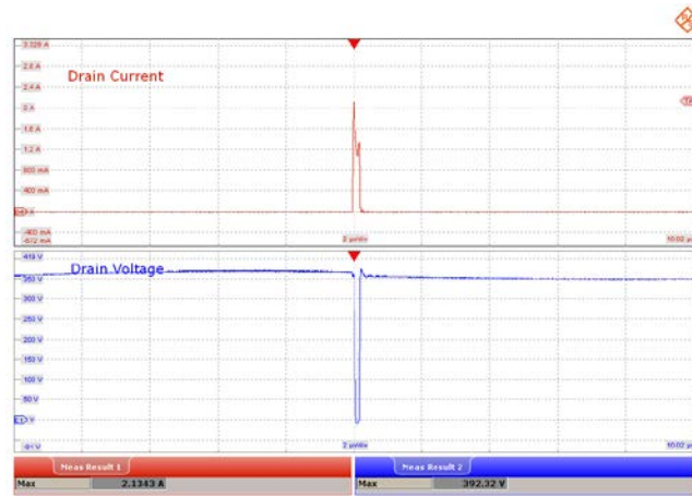
Figure 58 – 265 VAC, Output Short. Upper: I_{DRAIN} , 400 mA / div. Lower: V_{DRAIN} , 50 V / div., 2 \mu s / div. Peak I_{DRAIN} : 2.1343 A. Peak V_{DRAIN} : 392.32 V.
