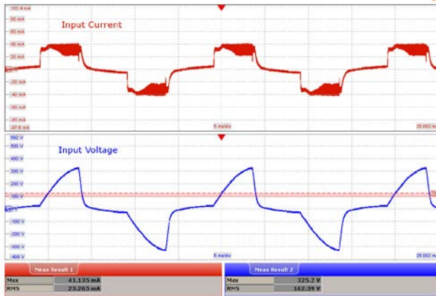
Figure 81 – 90° Conduction Angle. Upper: I_{IN} , 20 mA / div. Lower: V_{IN} , 100 V / div., 5 ms / div. Peak V_{IN} : 325.2 V. V_{RMS} : 162.39 V
