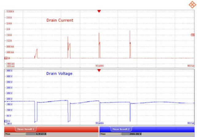
Figure 48 – 185 VAC, 30 V LED Load, Start-up. Upper: I_{DRAIN} , 400 mA / div. Lower: V_{DRAIN} , 50 V / div., 10 \mu s / div. Peak I_{DRAIN} : 1.913 A. Peak V_{DRAIN} : 268.36 V.
