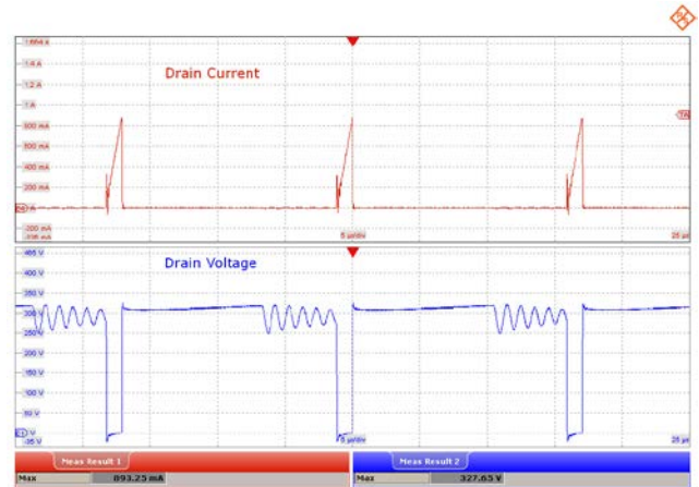
Figure 42 – 185 VAC, 30 V LED Load. Upper: I_{DRAIN} , 200 mA / div. Lower: V_{DRAIN} , 50 V / div., 5 \mu s / div. Peak I_{DRAIN} : 774.64 mA. Peak V_{DRAIN} : 260.45 V.
