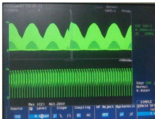
Figure 88 – 230 VAC, 50 Hz, -1000, 90°. Upper: V_{DRAIN} , 200 V / div. Lower: V_{DRAIN} , 200 V / div. (Zoomed). Measured Peak Voltage = 463 V_{PK} .
