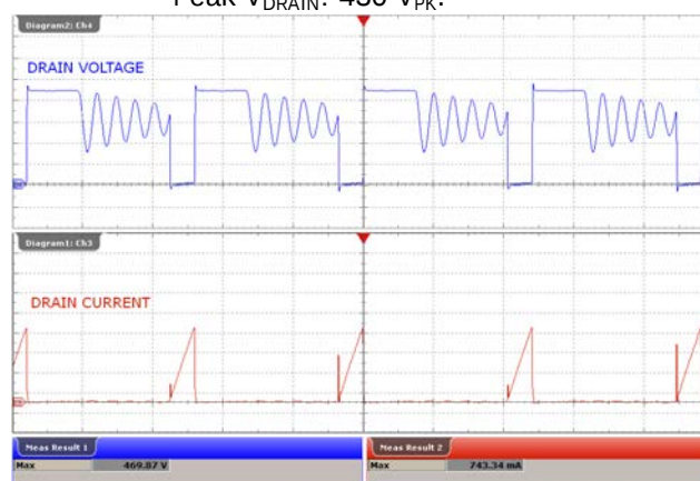
Figure 37 – 220 VAC, 141 V LED Load. Upper: V_{DRAIN} , 100 V / div., 4 \mu s / div. Lower: I_{DRAIN} , 200 mA / div. Peak I_{DRAIN} : 743 mA PK . Peak V_{DRAIN} : 470 V PK .
