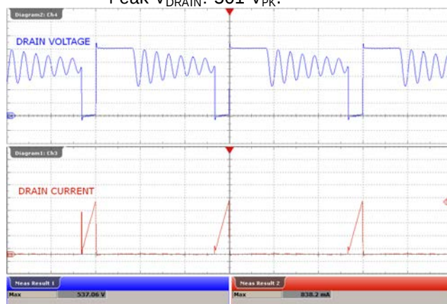
Figure 41 – 265 VAC, 141 V LED Load. Upper: V_{DRAIN} , 100 V / div., 4 μs / div. Lower: I_{DRAIN} , 200 mA / div. Peak I_{DRAIN} : 838 A PK . Peak V_{DRAIN} : 537 V PK .
