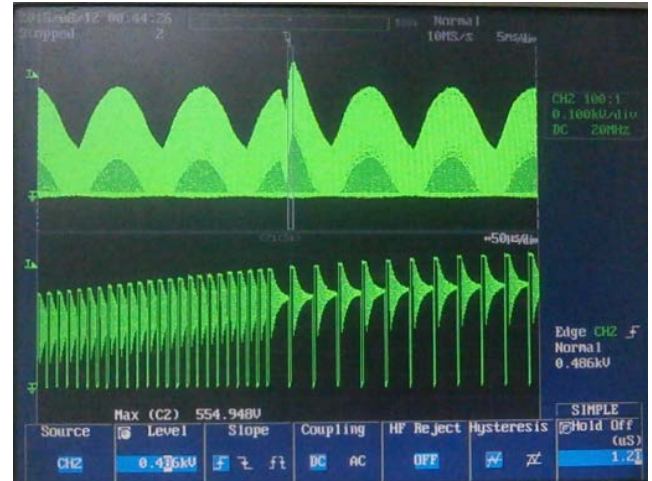
Figure 96 – 230 VAC, 50 Hz, -2500, 270°. Upper: V_{DRAIN} , 200 V / div. Lower: V_{DRAIN} , 200 V / div. (Zoomed). Measured Peak Voltage = 554 V_{PK} .
