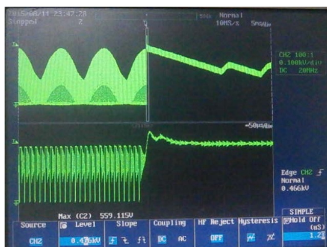
Figure 87 – 230 VAC, 50 Hz, +1000, 90°. Upper: V_{DRAIN} , 200 V / div. Lower: V_{DRAIN} , 200 V / div. (Zoomed). Measured Peak Voltage = 559 V_{PK} .
