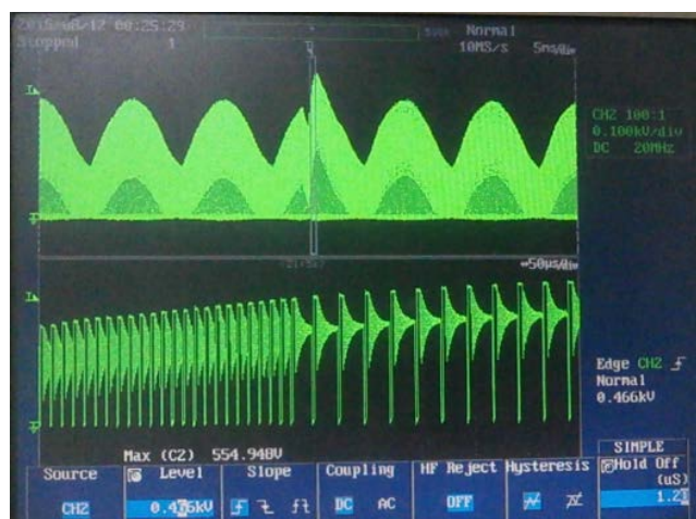
Figure 93 – 230 VAC, 50 Hz, +2500, 90°. Upper: V_{DRAIN} , 200 V / div. Lower: V_{DRAIN} , 200 V / div. (Zoomed). Measured Peak Voltage = 544 V_{PK} .
