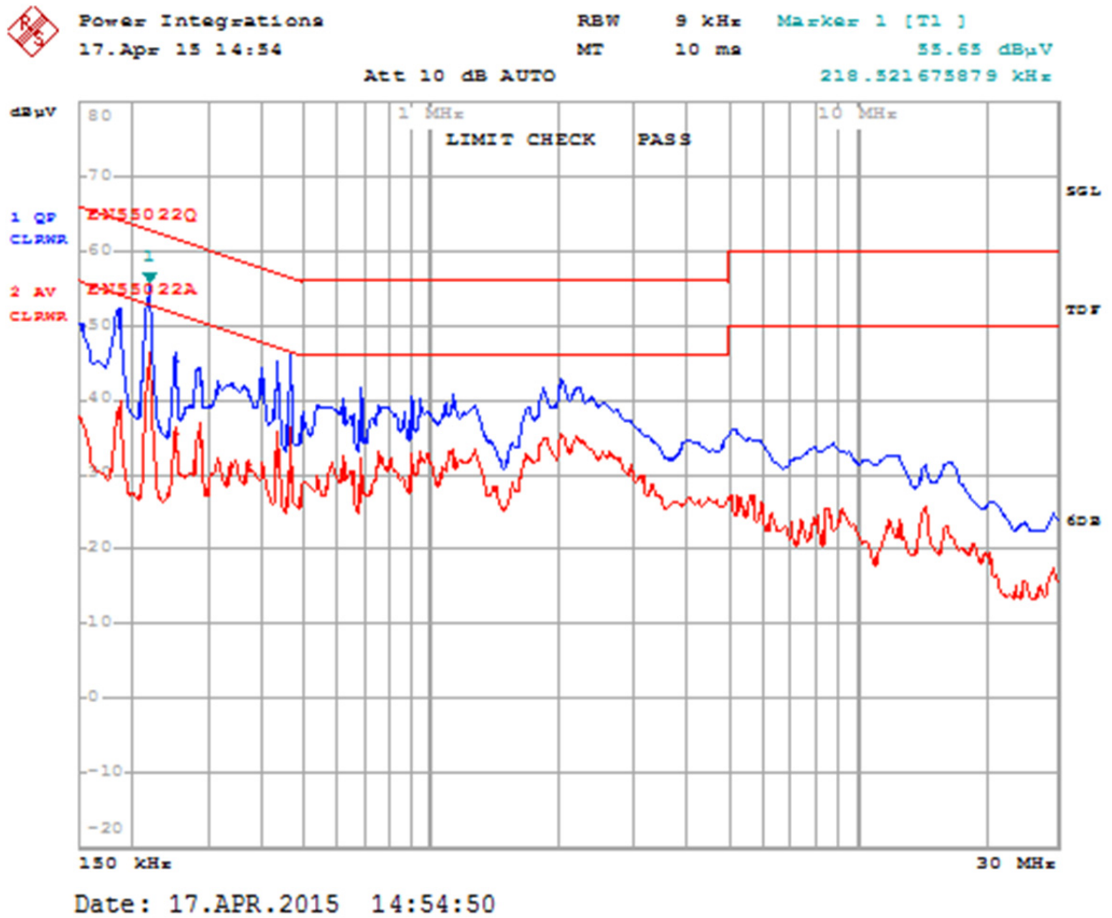
Figure 30 – QP (Blue) and AV (Red), 230 VAC, Full Load. Line to GND.
