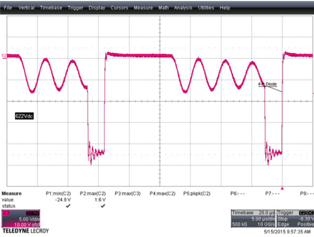
Figure 21 – 622 VDC, Full Load. V_{R(MAX)} = 24.9 V. C2: V_{OUT} for 4 V, 5 V / div.
