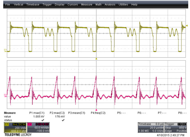
Figure 16 – 622 VDC, Peak Load. Upper: V_{CE} , 200 V / div. Lower: I_{CE} , 89 mA / div., 20 \mu s / div.
