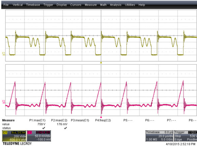
Figure 15 – 290 VAC, Peak Load. Upper: V_{CE} , 200 V / div. Lower: I_{CE} , 89 mA / div., 20 \mu s / div.
