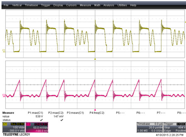
Figure 9 – 185 VAC, Full Load. Upper: V_{CE} , 100 V / div. Lower: I_{CE} , 89 mA / div., 20 \mu s / div.
