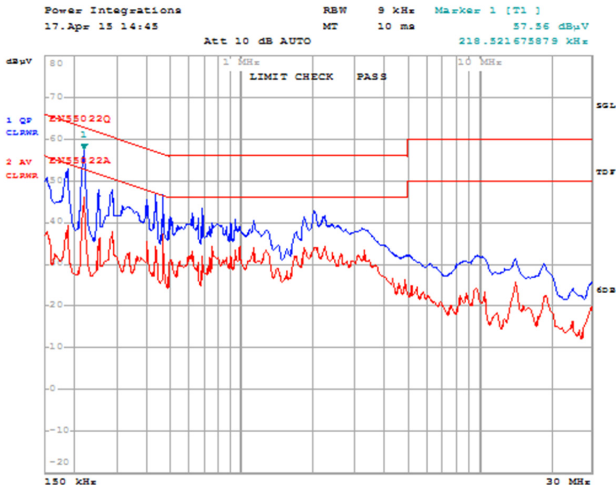
Figure 29 – QP (Blue) and AV (Red), 230 VAC, Full Load. Neutral to GND.
