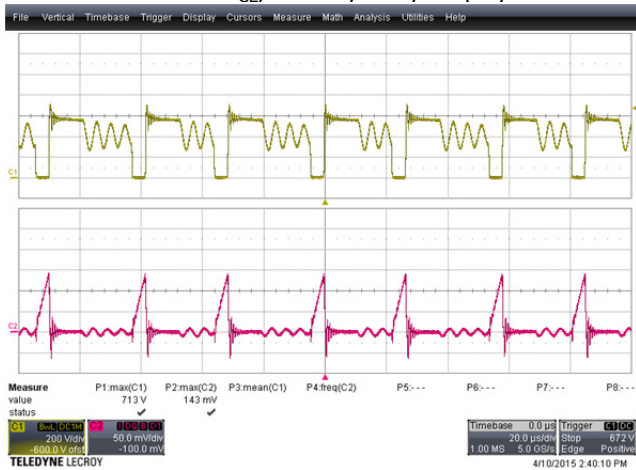
Figure 11 – 290 VAC, Full Load. Upper: V_{CE} , 200 V / div. Lower: I_{CE} , 89 mA / div., 20 \mu s / div.
