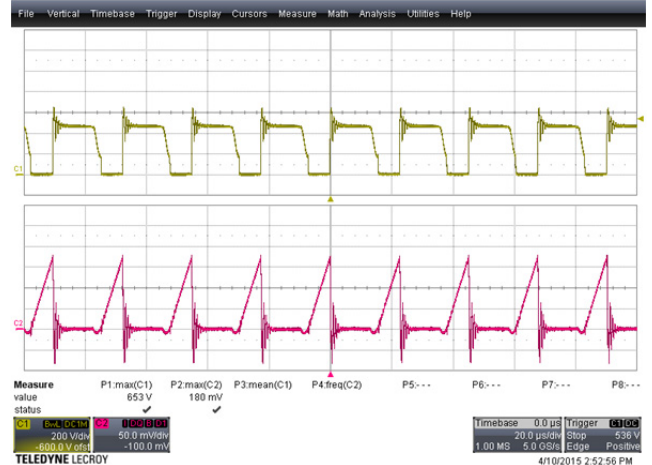
Figure 14 – 230 VAC, Peak Load. Upper: V_{CE} , 100 V / div. Lower: I_{CE} , 89 mA / div., 20 \mu s / div.
