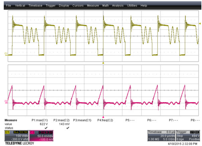
Figure 10 – 230 VAC, Full Load. Upper: V_{CE} , 100 V / div. Lower: I_{CE} , 89 mA / div., 20 \mu s / div.
