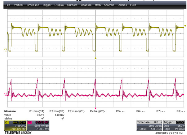
Figure 12 – 622 VDC, Full Load. Upper: V_{CE} , 200 V / div. Lower: I_{CE} , 89 mA / div., 20 \mu s / div.
