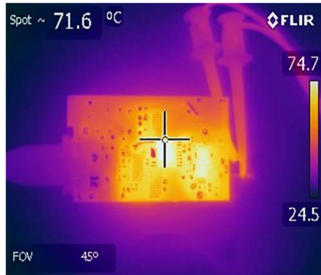
Figure 22 – InnoSwitch-CH Side. 230 VAC, 4 A Load. Ambient = 25.3 °C. InnoSwitch-CH, U1 = 78.2 °C. SR FET, Q1 = 73.1 °C. SR FET, Q2 = 73.9 °C. Clamp Resistor, R2 = 64 °C.
