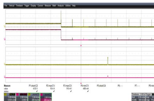
Figure 39 – Output Voltage and Current Waveforms. 265 VAC Input. Lower: I_{OUT} , 5 A / div. Upper: V_{OUT} , 2 V, 2 s / div.
