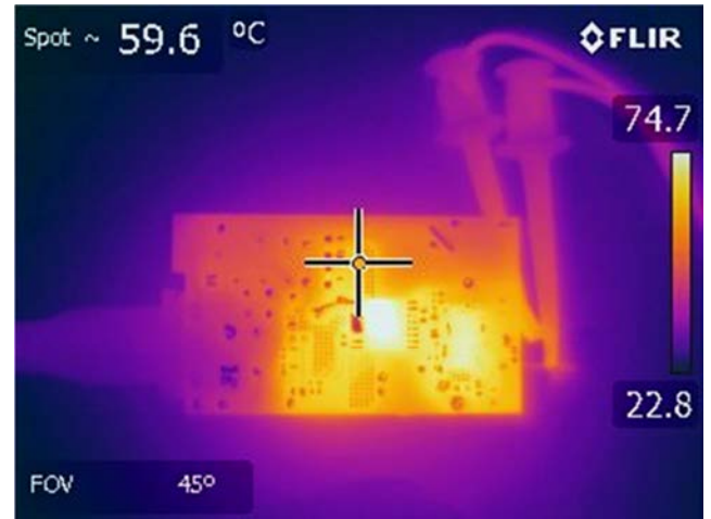
Figure 24 – InnoSwitch-CH Side. 265 VAC, 4 A Load. Ambient = 23.8 °C. InnoSwitch-CH, U1 = 78.8 °C. SR FET, Q1 = 71.4 °C. SR FET, Q2 = 72.7 °C. Clamp Resistor, R2 = 66.1 °C.
