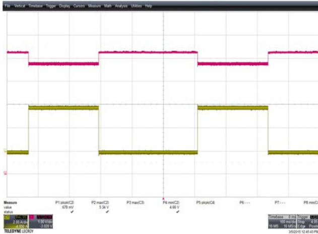
Figure 25 – Transient Response. 85 VAC, 0 - 4 A Load Step. V_{MIN} : 4.66 V, V_{MAX} : 5.34 V. Upper: I_{LOAD} , 2 A / div. Lower: V_{OUT} , 1 V, 100 ms / div.
