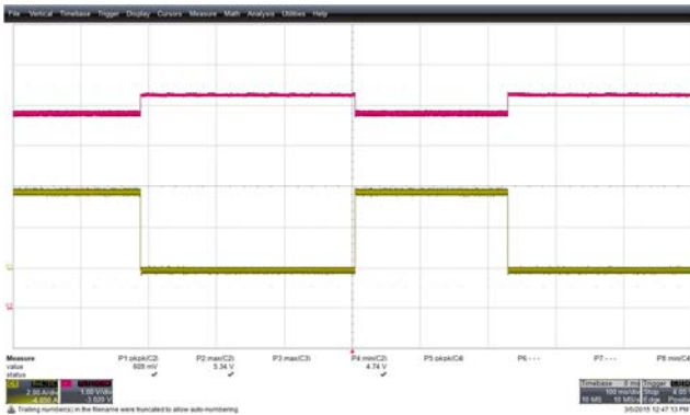
Figure 27 – Transient Response. 230 VAC, 0-4 A Load Step. V_{MIN} : 4.74 V, V_{MAX} : 5.34 V. Upper: I_{LOAD} , 2 A / div. Lower: V_{OUT} , 1 V, 100 ms / div.
