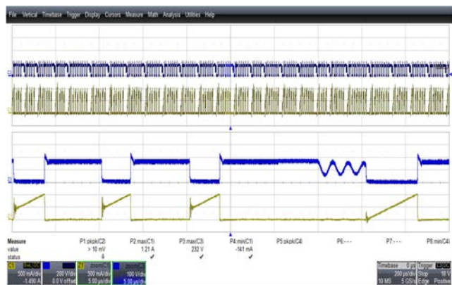
Figure 29 – Drain Voltage and Current Waveforms. 85 VAC, 4 A Load. Lower: I_{DRAIN} , 500 mA / div. Upper: V_{DRAIN} , 200 V, 200 \mu s, 5 \mu s / div.
