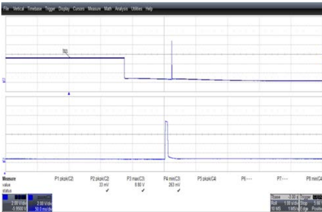
Figure 40 – Output Voltage Waveform. 85 VAC Input. V_{OUT} , 2 V, 1 s, 50 ms / div.
