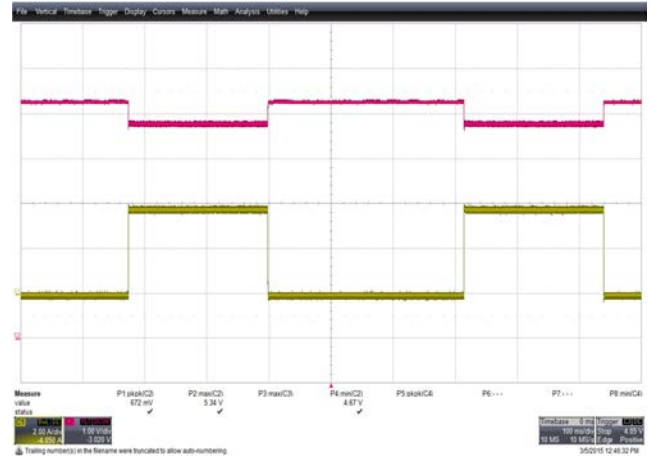
Figure 26 – Transient Response. 110 VAC, 0 - 4 A Load Step. V_{MIN} : 4.67 V, V_{MAX} : 5.34 V. Upper: I_{LOAD} , 2 A / div. Lower: V_{OUT} , 1 V, 100 ms / div.
