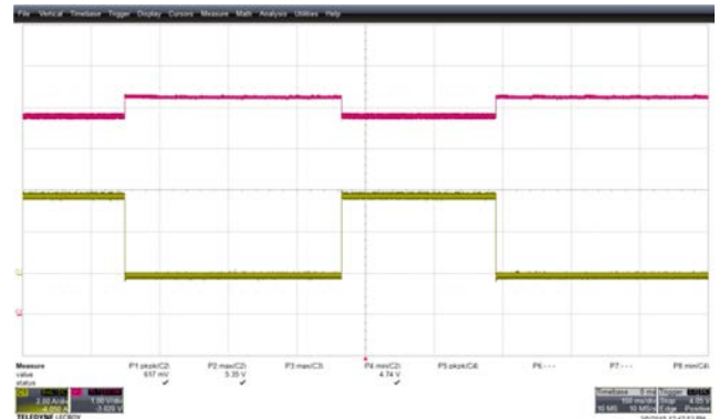
Figure 28 – Transient Response. 265 VAC, 0 - 4 A Load Step. V_{MIN} : 4.74 V, V_{MAX} : 5.35 V. Upper: I_{LOAD} , 2 A / div. Lower: V_{OUT} , 1 V, 100 ms / div.
