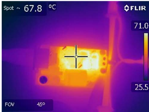
Figure 23 – Transformer Side. 265 VAC, 4 A Load. Ambient = 27.4 °C. Transformer, T1 = 67.3 °C. Input Capacitor, C1 = 28.5 °C. Input Capacitor, C2 = 51.5 °C. Bridge Rectifier, BR1 = 46.4 °C. Differential Choke, L3 = 43 °C.
