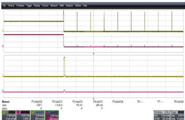
Figure 38 – Output Voltage and Current Waveforms. 85 VAC Input. Lower: I_{OUT} , 2 A / div. Upper: V_{OUT} , 2 V, 2 s / div.
