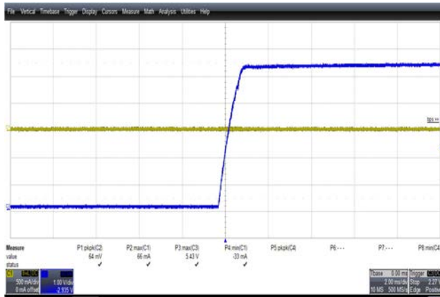
Figure 34 – Output Voltage and Current Waveforms. 85 VAC Input. Lower: I OUT , 500 mA / div. Upper: V OUT , 1 V, 2 ms / div.
