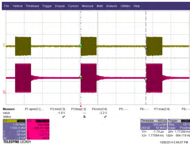
Figure 31 – LLC Stage Primary Voltage and Current, 90 VAC Input, CV Load, 0.5 A Current Limit, 8 V Load Setting. Upper: Current, 1 A / div. Lower: Voltage, 100 V, 500 µs / div.
