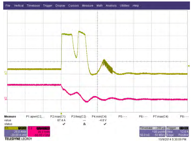
Figure 48 – Output Short-Circuit Test. Upper: LLC I_{OUT} , 20 A / div. Lower: LLC V_{OUT} , 20 V, 100 \mu s / div.
