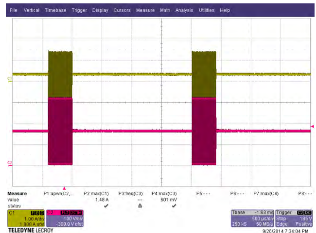
Figure 38 – LLC Stage Primary Voltage and Current, 115 VAC Input, CV Load, 0.5 A Current Limit, 0.5 V Load Setting. Upper: Current, 1 A / div. Lower: Voltage, 100 V, 500 \mu s / div.
