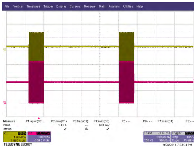
Figure 37 – LLC Stage Primary Voltage and Current, 115 VAC Input, CV Load, 0.5 A Current Limit, 2 V Load Setting. Upper: Current, 1 A / div. Lower: Voltage, 100 V, 500 \mu s / div.
