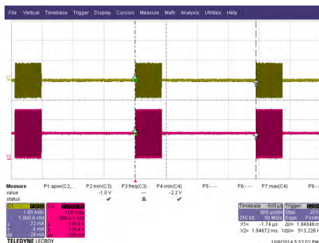
Figure 34 – LLC Stage Primary Voltage and Current, 90 VAC Input, CV Load, 0.5 A Current Limit, 0.5 V Load Setting. Upper: Current, 1 A / div. Lower: Voltage, 100 V, 500 \mu s / div.
