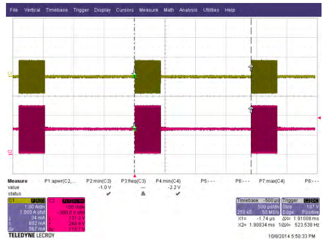
Figure 32 – LLC Stage Primary Voltage and Current, 90 VAC Input, CV Load, 0.5 A Current Limit, 4 V Load Setting. Upper: Current, 1 A / div. Lower: Voltage, 100 V, 500 µs / div.
