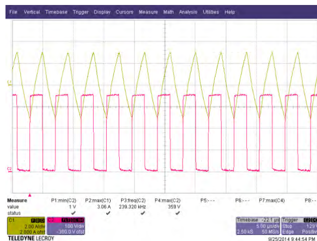
Figure 30 – LLC Stage Primary Voltage and Current, 132 VAC Input, CV Load, 8 A Current Limit, 8 V Load Setting. Upper: Current, 2 A / div. Lower: Voltage, 100 V, 5 \mu s / div.
