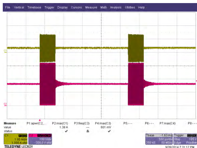
Figure 35 – LLC Stage Primary Voltage and Current, 115 VAC Input, CV Load, 0.5 A Current Limit, 8 V Load Setting. Upper: Current, 1 A / div. Lower: Voltage, 100 V, 500 \mu s / div.
