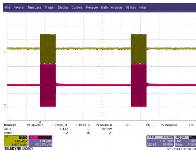
Figure 36 – LLC Stage Primary Voltage and Current, 115 VAC Input, CV Load, 0.5 A Current Limit, 4 V Load Setting. Upper: Current, 1 A / div. Lower: Voltage, 100 V, 500 \mu s / div.
