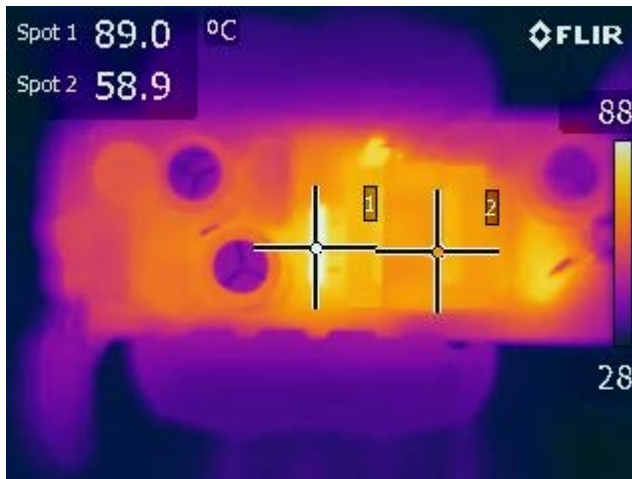
Figure 16 – 90 VAC, Thermal, Top Side. SPOT1 (U1): 89.0 °C. SPOT2 (T1): 58.9 °C.
