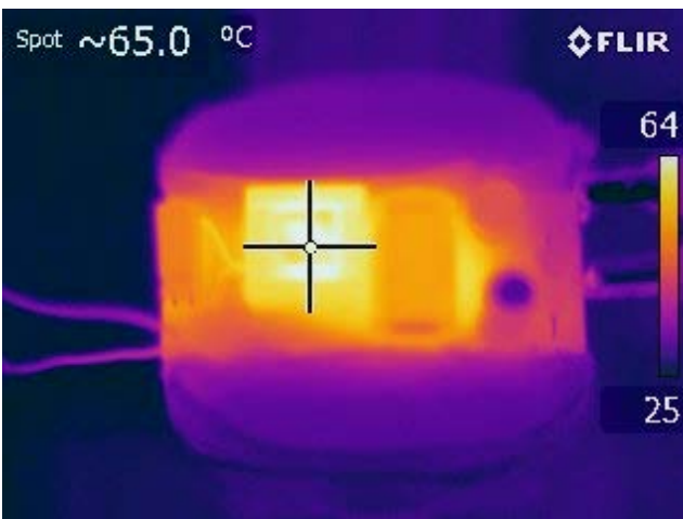
Figure 15 – 265 VAC, Thermal, Top Side. SPOT1 (T1): 65.0 °C.
