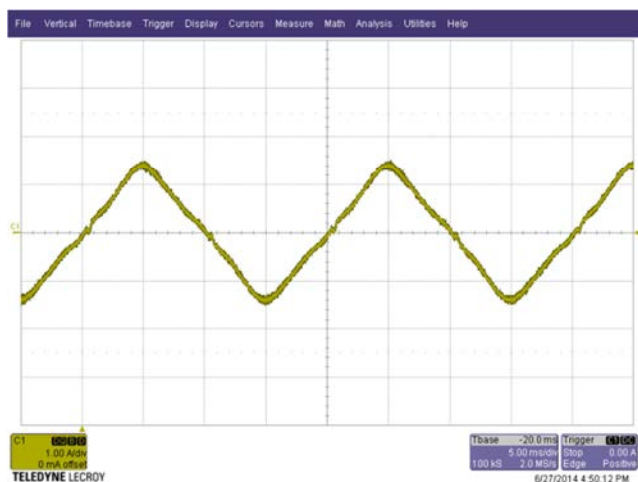
Figure 29 – Input Current, 230 VAC, 100% Load, 1 A, 5 ms / div.
