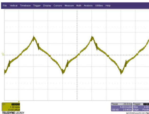
Figure 30 – Input Current, 264 VAC, 100% Load, 1 A, 5 ms / div.
