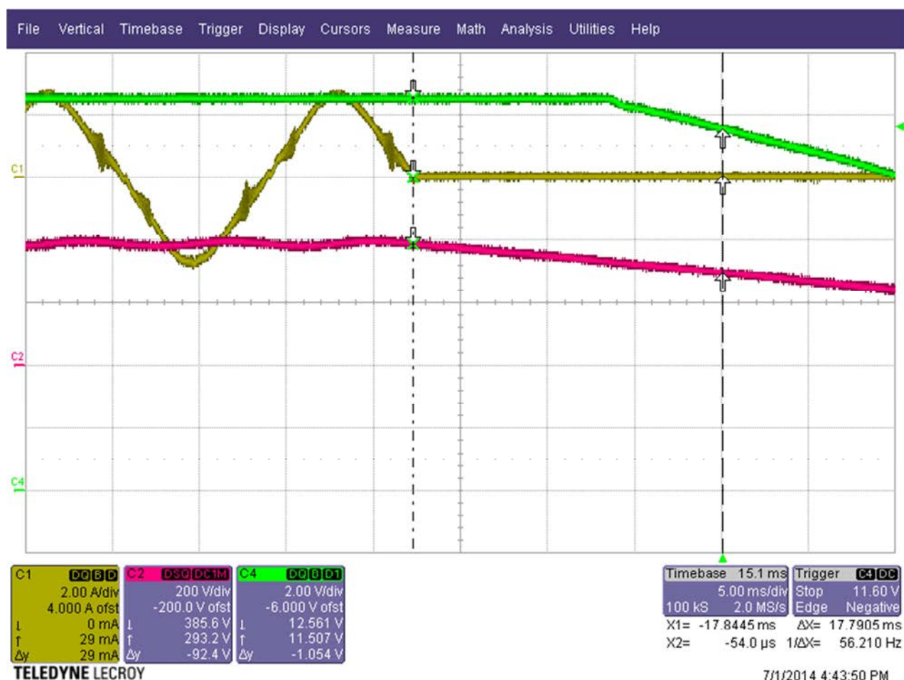
Figure 67 – DER-428 Hold-up Time using 120 \mu\text{F} Bulk Capacitor (C15), 115 VAC Input, 100% Load.
