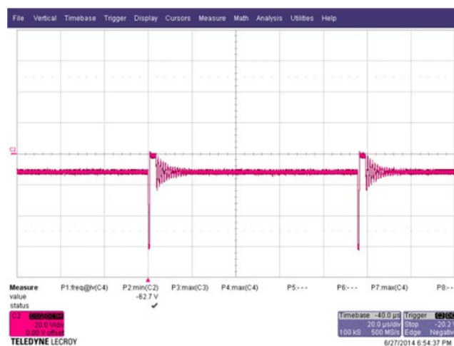
Figure 36 – +12 V Standby Output Rectifier (D10) Reverse Voltage, 100% Load, 230 VAC Input, Main / PFC Disabled. 20 V, 20 \mu s / div.
