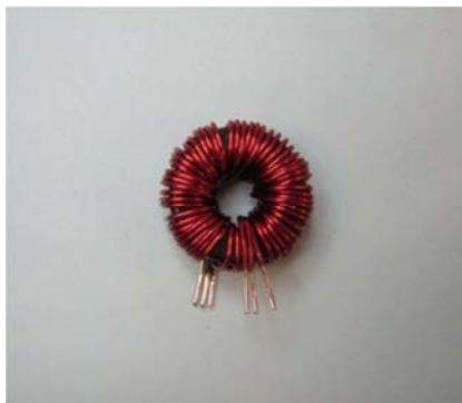
Figure 15 – Finished Part, Front View. Tin Leads to within ~ 1/2" of Toroid Body.
