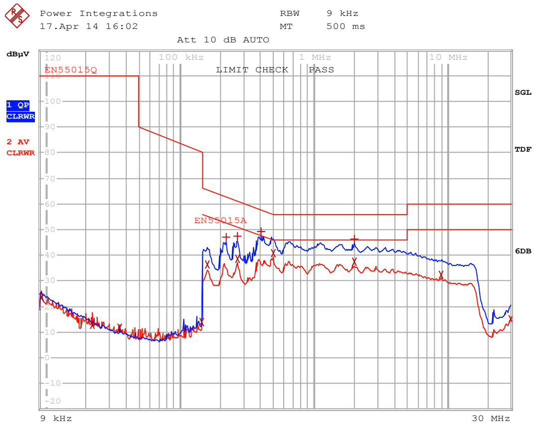
Figure 27 – Conducted EMI, Maximum Steady-State Load, 230 VAC, 60 Hz, and EN55015 B Limits. Unit on Top of Copper Plane that is Connected to Earth.
