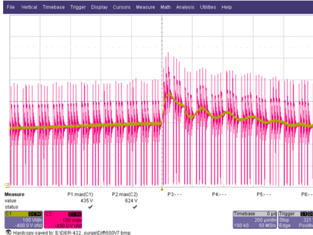
Figure 67 – Differential Surge of 2.5 kV, 230 VAC at 90°. Yellow: V_{BULK} , 100 V / div. Red: V_{DS} , 100 V / div. Time Scale: 1 ms / div.
