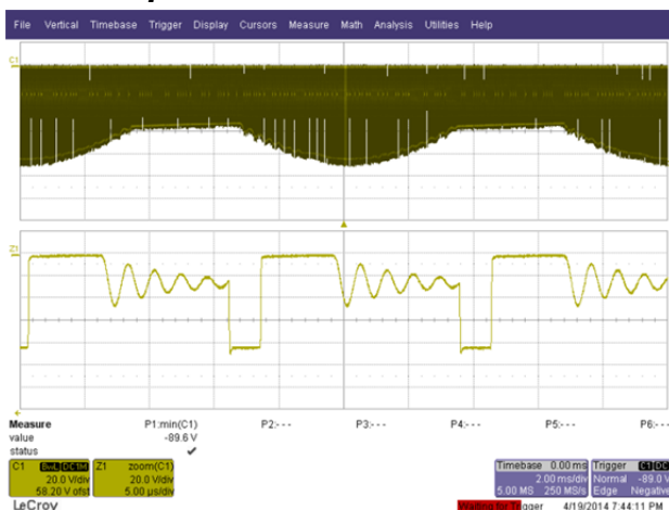
Figure 45 – 190 VAC Input and Full Load. Upper: V_{DIODE} , 0.2 A / div. Lower, Zoom: V_{DIODE} , 20 V / div. Time Scale: 2 ms / div. Zoom Time Scale: 5 \mu s / div.
