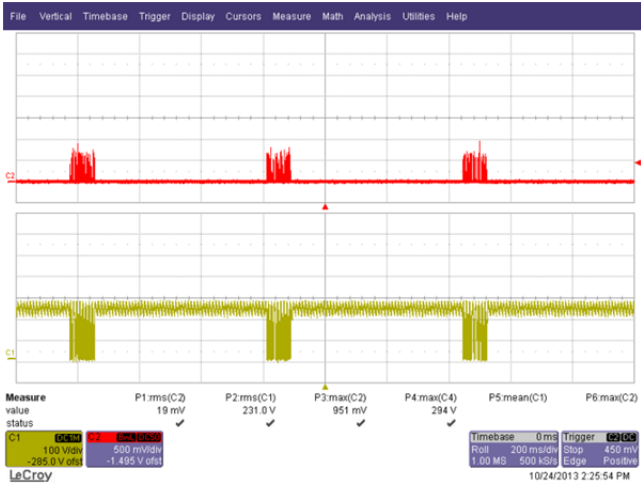
Figure 39 – 185 VAC, 50 Hz Output Short Condition. Upper: I_{DRAIN} , 500 mA / div. Lower: V_{DRAIN} , 100 V, 200 ms / div.
