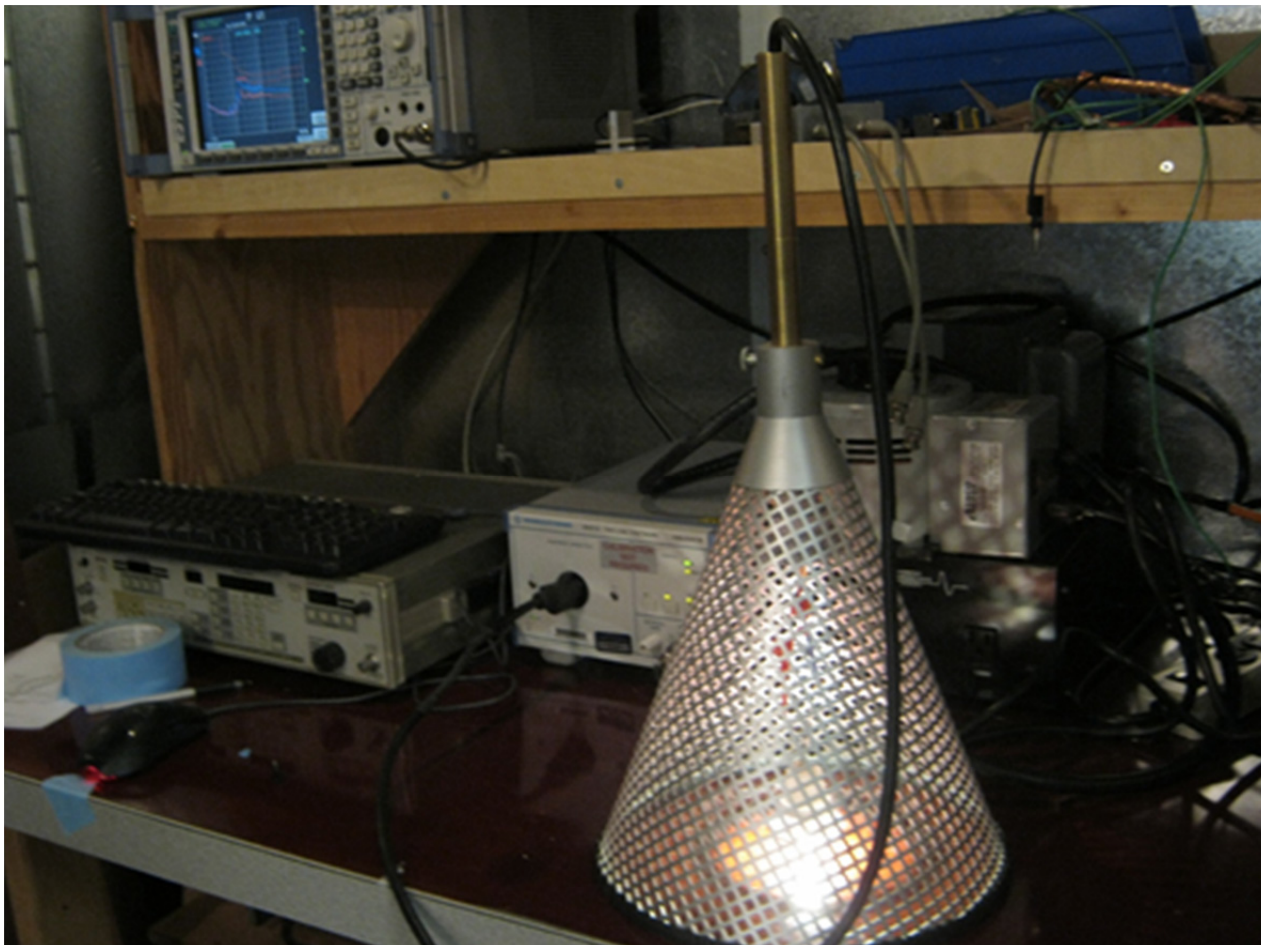
Figure 44 – Conducted EMI Test Set-up.
