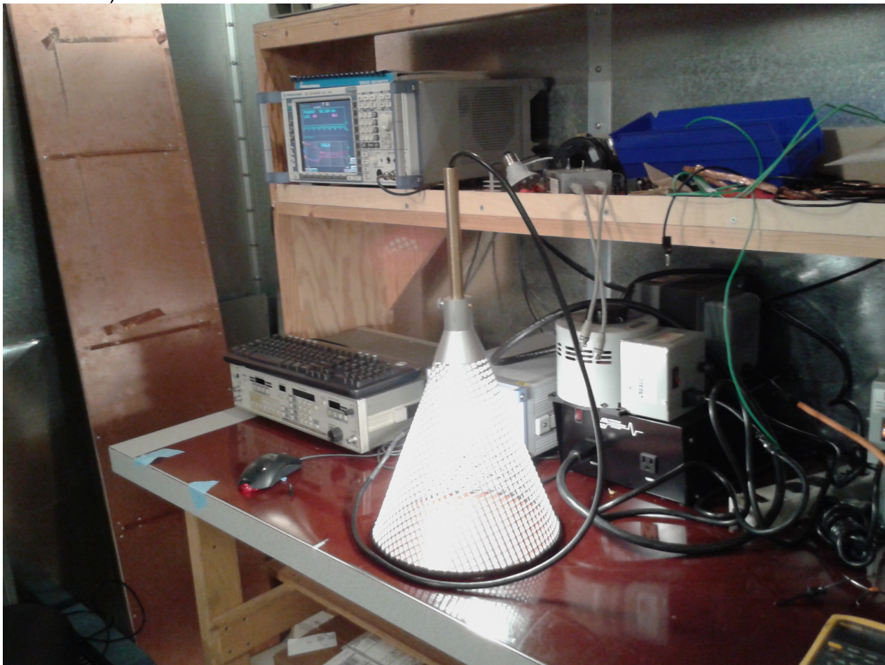
Figure 39 – Conducted Emissions Measurement Set-up.
