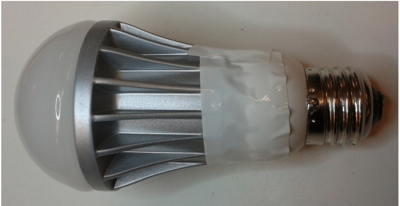
Figure 50 – LED Driver is Enclosed in Temporary A19 Housing that is Mounted in the Conical Ground Plane.
