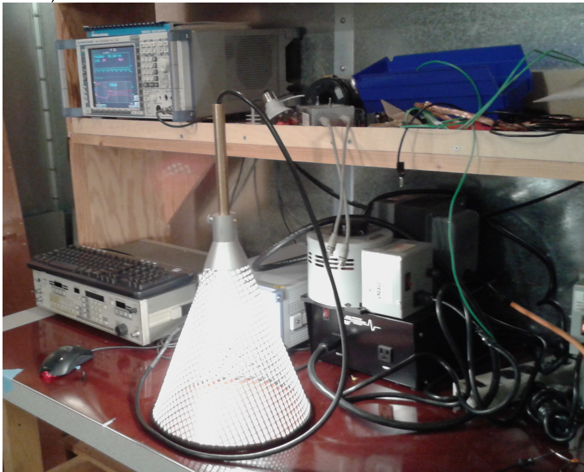
Figure 49 – Conducted Emissions Measurement Set-up Showing Conical Ground Plane Inside which UUT was Mounted.
