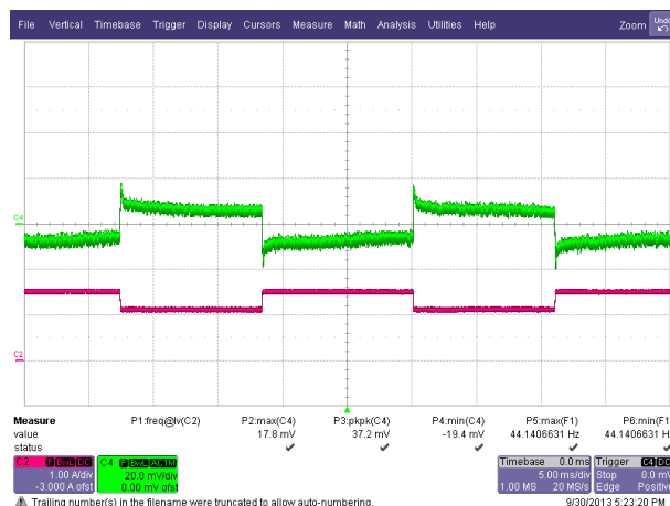
Figure 56 – Output Transient Response 75%-100%-75%, 5 ms / div. Upper: V_{OUT} , 20 mV / div. Lower: I_{LOAD} , 1 A / div.
