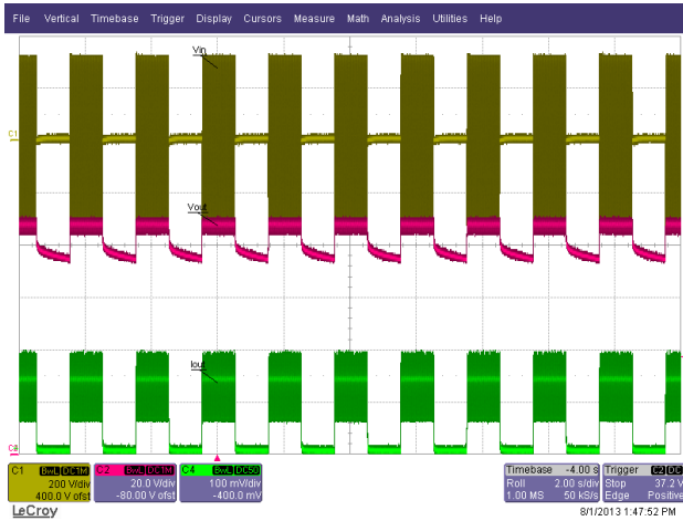
Figure 49 – Line Sag Test at 230 - 0 V at 1 s Interval. Ch1: V_{IN} , 200 V / div. Ch2: V_{OUT} , 20 V / div. Ch4: I_{OUT} , 100 mA / div. Time Scale: 2 s / div.
