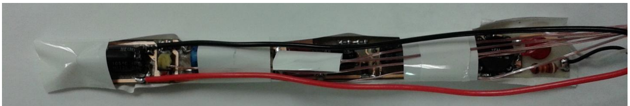
Figure 18 – Thermal Unit with Thermocouple Set-up.
