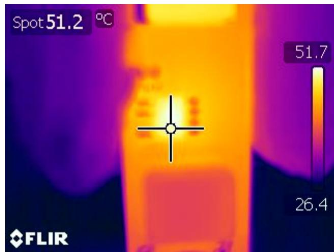
Figure 20 – LYT0006D Device Temperature (°C).
