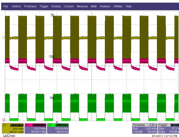
**Figure 49 – Line Sag Test at 230 - 0 V at 1 s Interval.**
