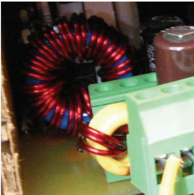
Figure 58 – Main Output Choke L1, Visible Light View.
