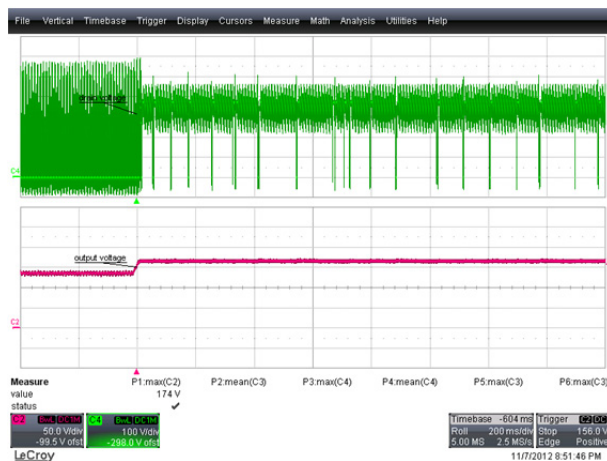
Figure 38 – 265 VAC 50 Hz, Open Load. Upper: V_{DRAIN} , 100 V / div. Lower: V_{OUT} , 50 V, 200 ms / div.
