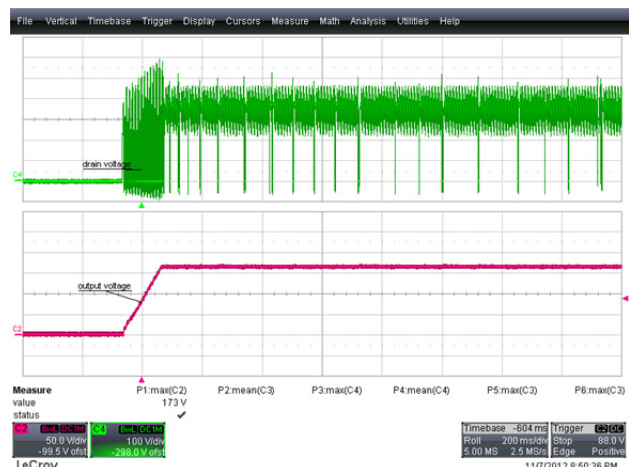
Figure 39 – 265 VAC 50 Hz, Open Load Start-up Upper: V_{DRAIN} , 100 V / div. Lower: V_{OUT} , 50 V, 200 ms / div.
