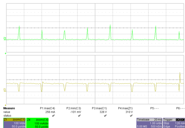
Figure 41 – 90 VAC, 60 Hz Output Short Condition. Upper: I_{DRAIN} , 100 mA / div. Lower: V_{DRAIN} , 100 V, 10 \mu s / div.
