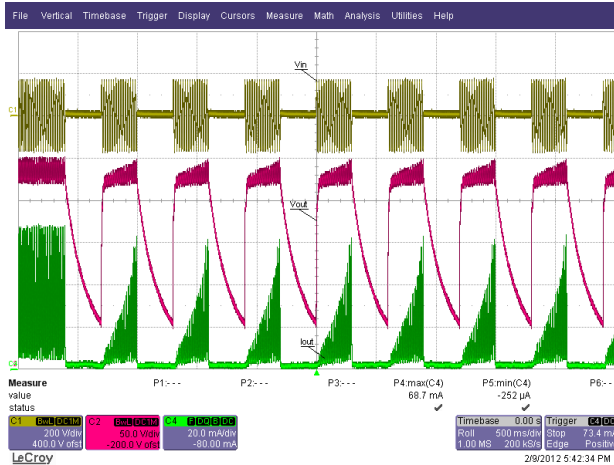
Figure 51 – 115 VAC / 50 Hz, 300 ms On – 300 ms Off. Load: 230 V LED String. Ch1: V_{IN} , 200 V / div. Ch2: V_{OUT} , 50 V / div. Ch4: I_{OUT} , 20 mA / div. Time Scale: 0.5 s / div.
