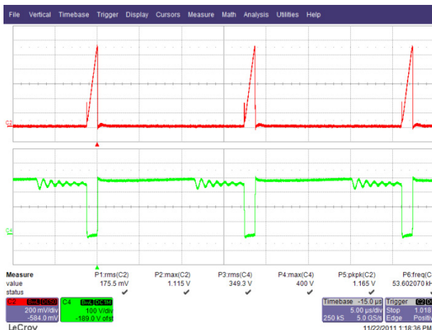
Figure 40 – 265 VAC, 50 Hz. Upper: I_{DRAIN} , 200 mA / div. Lower: V_{DRAIN} , 100 V, 5 ms / div.
