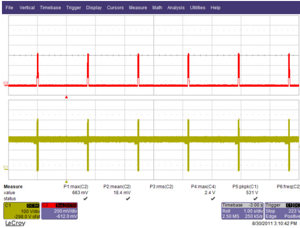
Figure 69 – 230 VAC, 50 Hz Output Short Condition. Upper: I_{OUT} , 200 mA / div. Lower: V_{DRAIN} , 100 V, 1 s / div.
