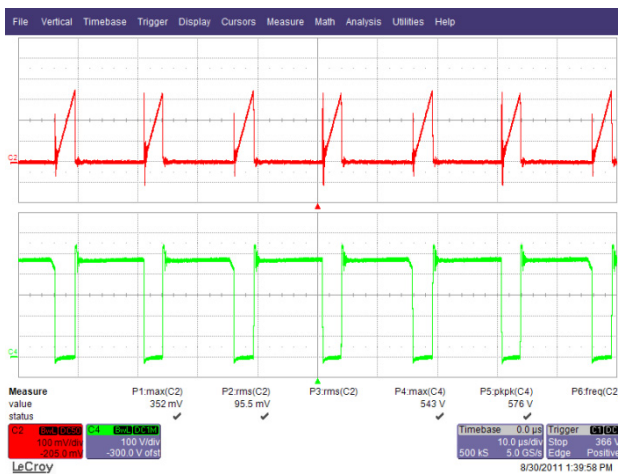
Figure 60 – 265 VAC, 50 Hz. Upper: I_{DRAIN} , 0.1 A / div. Lower: V_{DRAIN} , 100 V / div., 10 \mu s / div.
