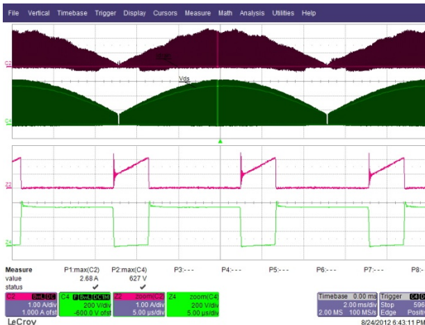
Figure 20 – 277 VAC 50 Hz, Full Load. Upper: I_{DRAIN} , 1 A / div. Lower: V_{DRAIN} , 200 V, 2 ms / div.
