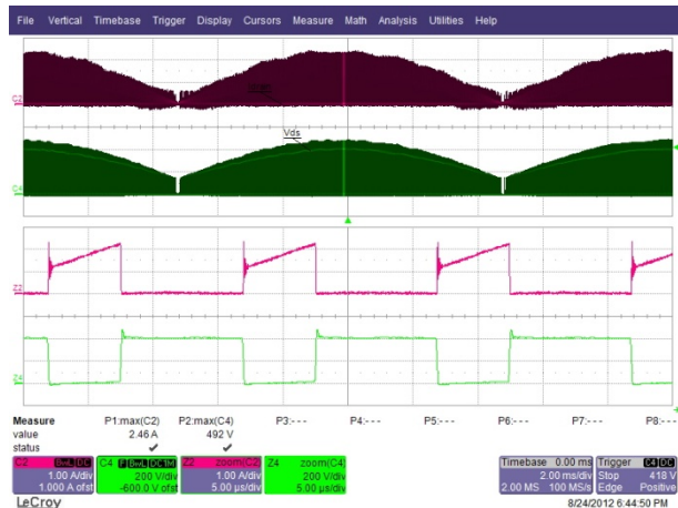
Figure 19 – 184 VAC 50 Hz, Full Load. Upper: I_{DRAIN} , 1 A / div. Lower: V_{DRAIN} , 200 V, 2 ms / div.
