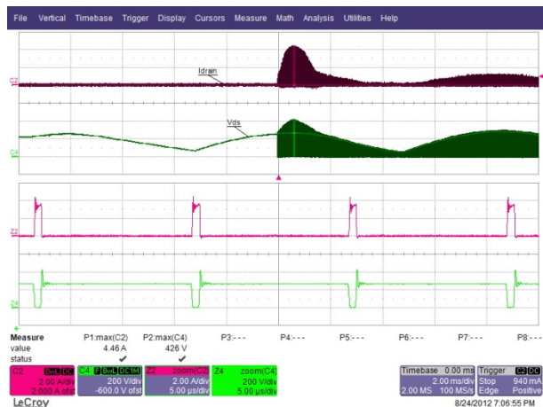
Figure 21 – 184 VAC 50 Hz., Full Load Start-up. Upper: I_{DRAIN} , 2 A / div. Lower: V_{DRAIN} , 200 V, 2 ms / div.
