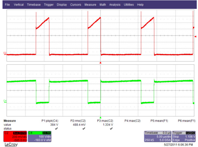
Figure 24 – 180 VAC 50 Hz, Full Load. Upper: I_{DRAIN} , 200 mA / div. Lower: V_{DRAIN} , 100 V, 5 \mu s / div.
