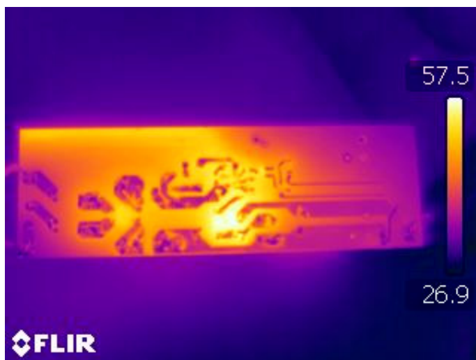
Figure 40 – Bottom-Side Thermal Measurements.
