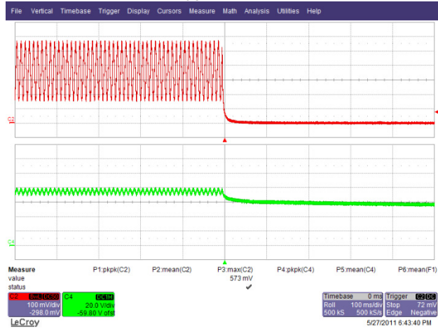
Figure 36 – 265 VAC 50 Hz, Output Fall. Upper: I_{OUT} , 100 mA / div. Lower: V_{OUT} , 20 V, 100 ms / div.
