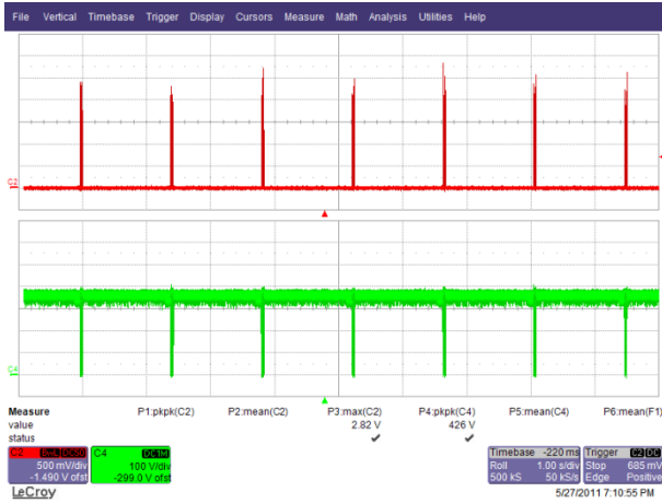
Figure 37 – 265 VAC 50 Hz, Output Short. Upper: I_{DRAIN} , 0.5 A / div. Lower: V_{DRAIN} , 100 V, 500 ms / div.
