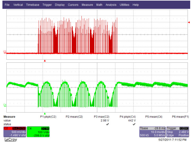
Figure 38 – 265 VAC 50 Hz, Output Short. Upper: I_{DRAIN} , 0.5 A / div. Lower: V_{DRAIN} , 100 V, 5 ms / div.
