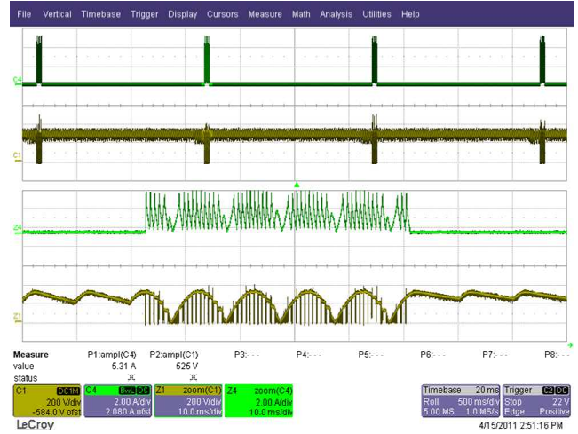
Figure 28 – 265 VAC, Full Load. Upper: I_{OUT} , 2 A / div. Lower: V_{DRAIN} , 200 V, 500 ms / div.
