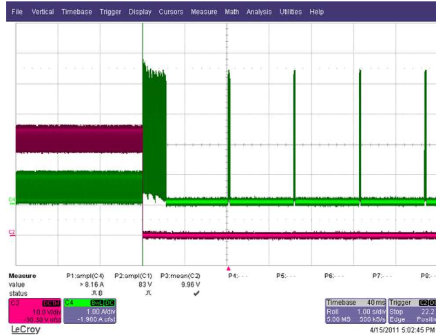
Figure 29 – 110 VAC, Full Load. Upper: I_{OUT} , 1 A / div. Lower: V_{DRAIN} , 10 V, 1 s / div.
