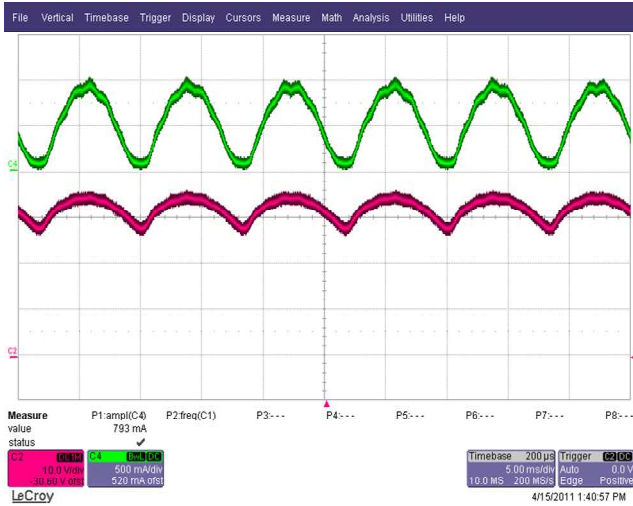
Figure 21 – 90 VAC, Full Load. Upper: I_{RIPPLE} , 0.5 A / div. Lower: V_{OUT} , 10 V, 5 ms / div.
