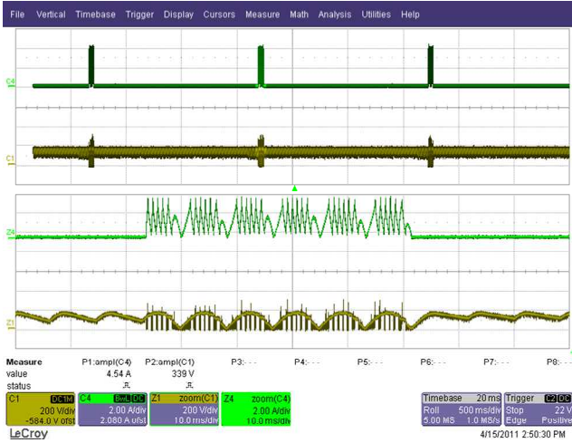
Figure 27 – 90 VAC, Full Load. Upper: I_{OUT} , 2 A / div. Lower: V_{DRAIN} , 200 V, 500 ms / div.
