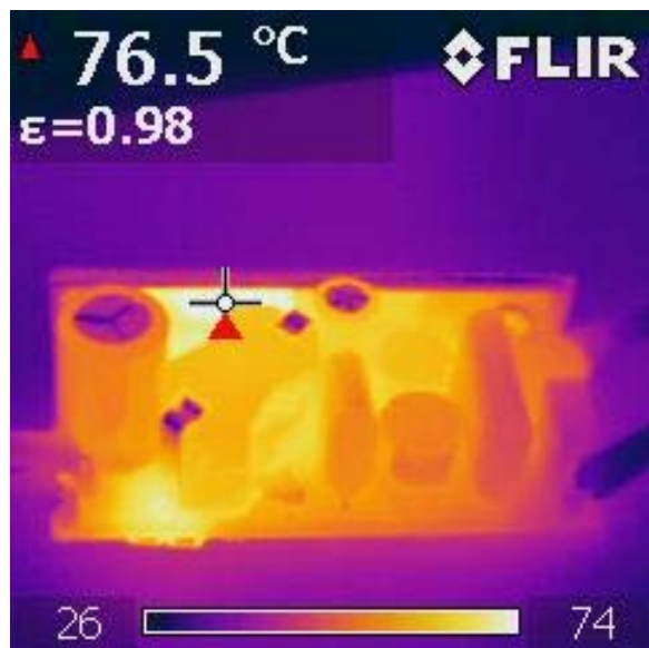
Figure 34 – 90 VAC 60 Hz, Thermals. Top Side. Device: U1 - LNK406EG
