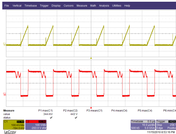
Figure 23 – 185 VAC, Full Load. Upper: I_{DRAIN} , 0.1 A / div. Lower: V_{DRAIN} , 100 V, 10 \mu s / div.
