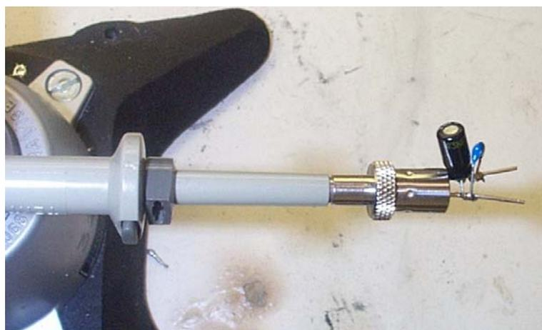
**Figure 27** – Oscilloscope Probe with Probe Master ([www.probemaster.com](http://www.probemaster.com)) 4987A BNC Adapter (modified with wires for ripple measurement and two parallel decoupling capacitors added).
