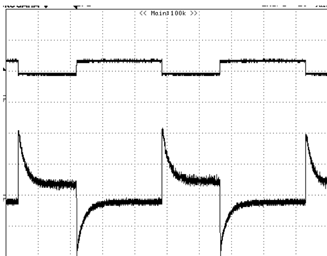
Figure 19 – Transient Response, 115 VAC, 50-100-50% Load Step. Top: Load Current, 0.5 A/div. Bottom: Output Voltage 200 mV, 10 ms / div.
