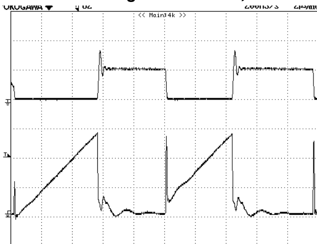
Figure 13 – 85 VAC, Full Load. Upper: V_{DRAIN} , 200 V / div. Lower: I_{DRAIN} , 50 mA / div, 2 \mu s / div.
