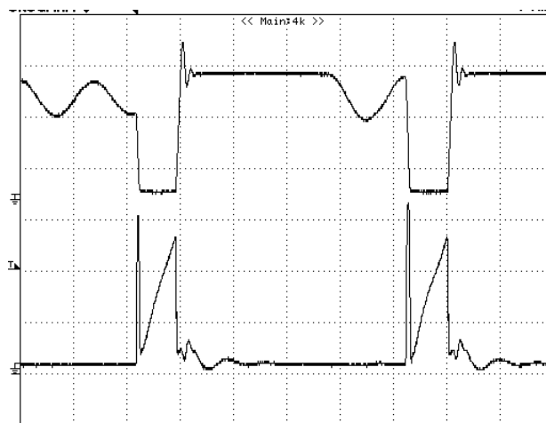
Figure 14 – 265 VAC, Full Load. Upper: V_{DRAIN} , 200 V / div. Lower: I_{DRAIN} , 50 mA / div, 2 \mu s / div.
