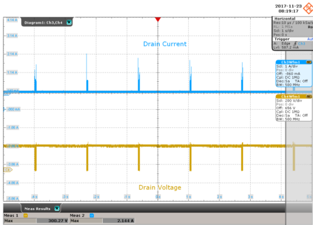
Figure 65 – 180 VAC 50 Hz, Output Shorted. Upper: I_{DRAIN} , 1 A / div. Lower: V_{DRAIN} , 200 V / div., 1 s / div. P_{IN} Average: 176 mW.
