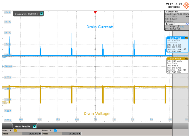
Figure 65 – 180 VAC 50 Hz, Output Shorted. Upper: I_{DRAIN} , 1 A / div. Lower: V_{DRAIN} , 200 V / div., 1 s / div. P_{IN} Average: 176 mW.
