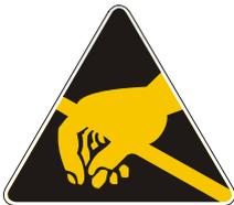
Any handling of IGBT modules or drivers is subject to the general specifications for protecting electrostatic-sensitive devices according to international standard IEC 60747-1, Chapter IX or European standard EN 100015 (i.e. the workplace, tools, etc. must comply with these standards).
