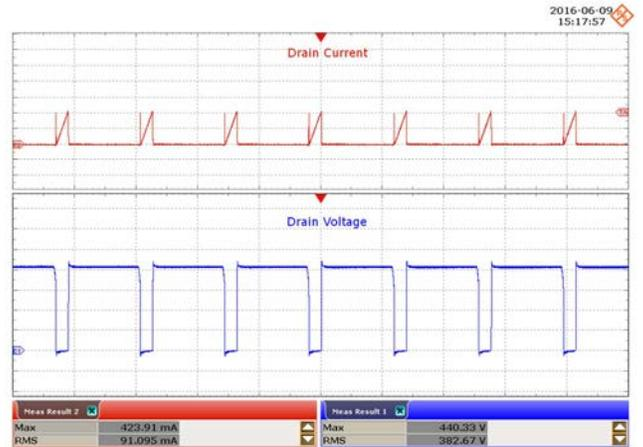
**Figure 41** – 300 VAC, 60 V LED Load.
