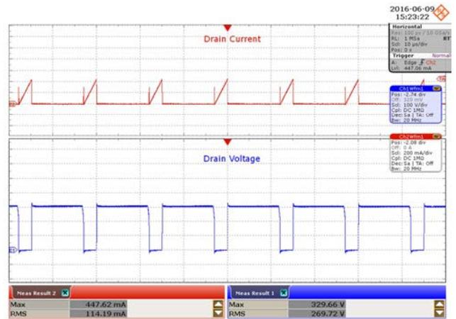
**Figure 39** – 230 VAC, 60V LED Load.
