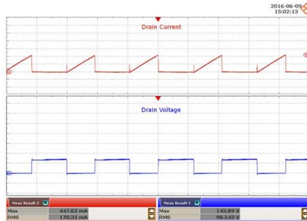
**Figure 37** – 115 VAC, 60 V LED Load.
