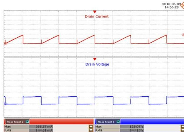
**Figure 35** – 90 VAC, 60 V LED Load.
