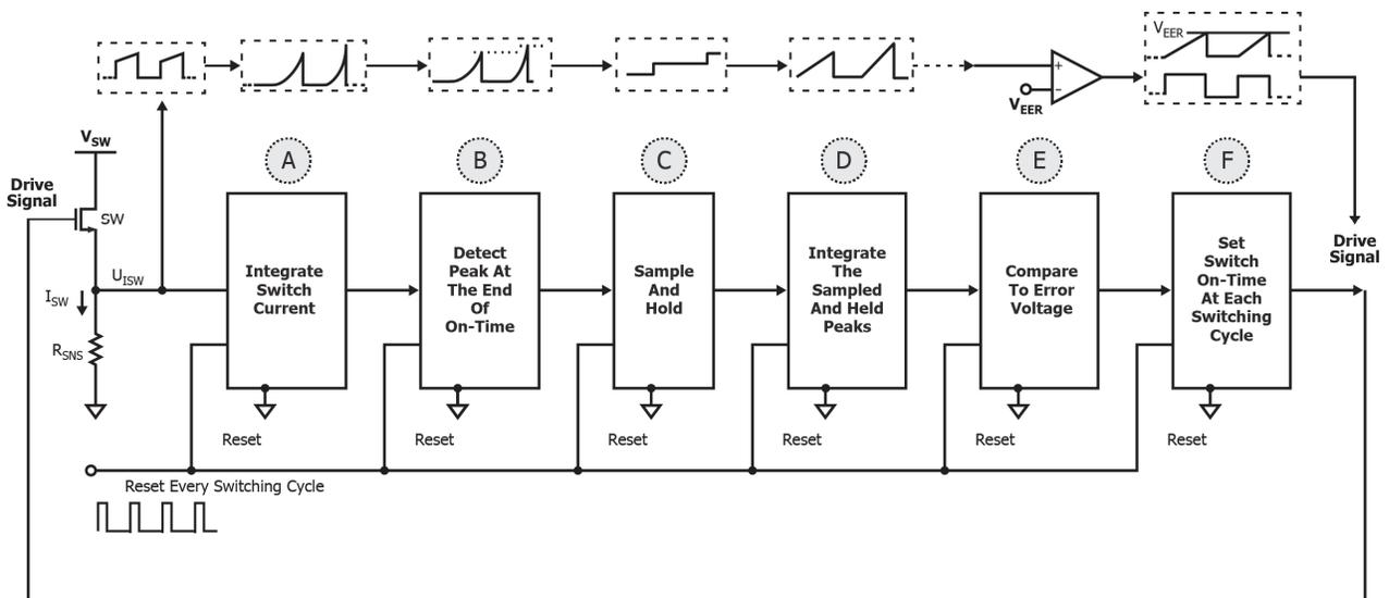
Figure 2. Summarized steps of PFC control blocks required for the HF process of switching current inside the controller.
