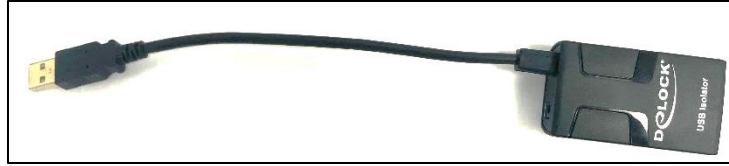
Figure 33 – Delock USB Isolator (Part Number: 62588).
