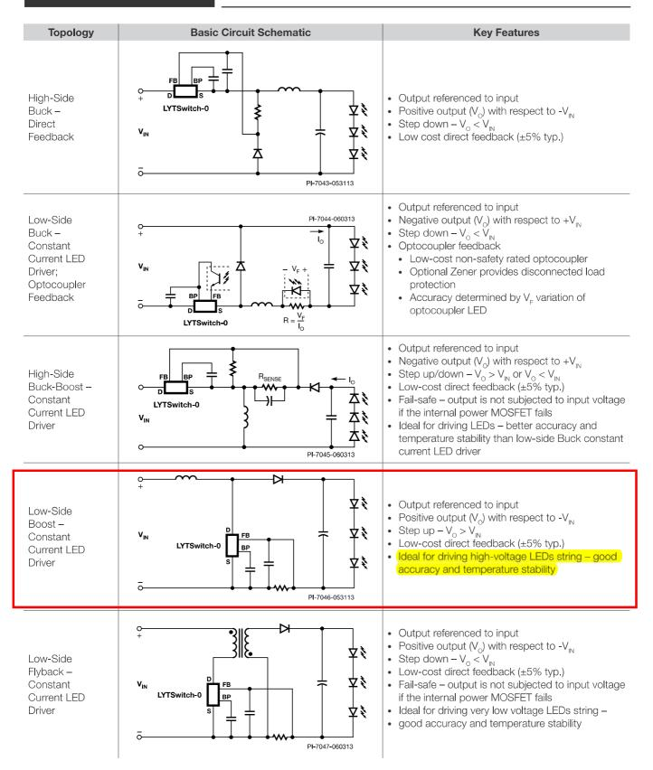
Table 2. Common Circuit Configurations Using LYTSwitch-0 for Driving LEDs.
