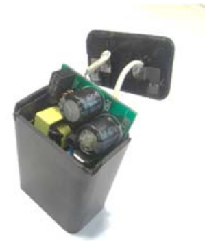
Test set up with UUT inside a simulated casing
