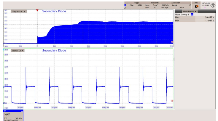
Figure 41 – 115 VAC 60 Hz. CH1: Sec Diode, 10 V / div., 5 ms / div. Zoom: 5 \mu s / div. Freewheel Diode Voltage (MAX) = 59.5 V
