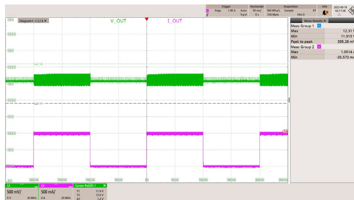
Figure 86 – 265 VAC 50 Hz. CH3: V_{OUT} , 500 mV / div., 50 ms / div. CH4: I_{OUT} , 500 mA / div., 50 ms / div. V_{OUT} : V_{MAX} : 12.3 V V_{MIN} : 11.9 V
