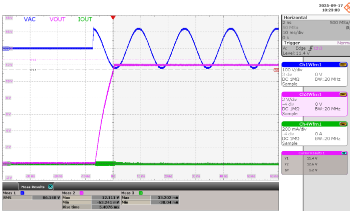
Figure 56 – 85 VAC 60 Hz. CH1: Input Voltage, 100 V / div., 10 ms / div. CH3: Vout, 2 V / div., 10 ms / div. CH4: Iout, 200 mA / div., 10 ms / div. V 0 Rise Time = 5.41 ms V MAX = 12.1 V
