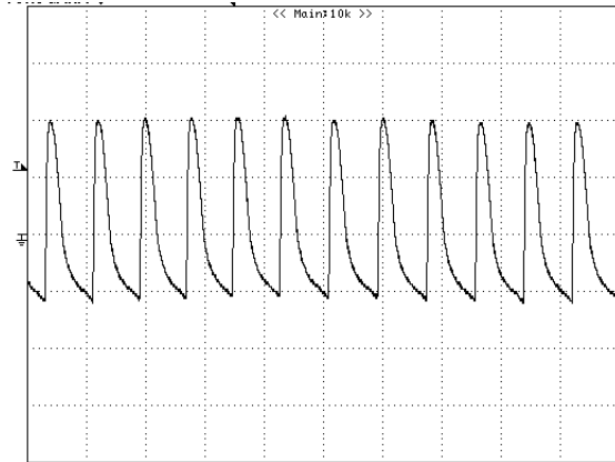
Figure 32 – Ripple, 85 VAC, Full Load, 20 mV, 20 μs / div.
