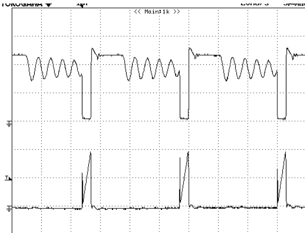
Figure 17 – 265 VAC, Full Load. Upper: V_{DRAIN} , 200 V / div. Lower: I_{DRAIN} , 100 mA / div. 5 us / div.
