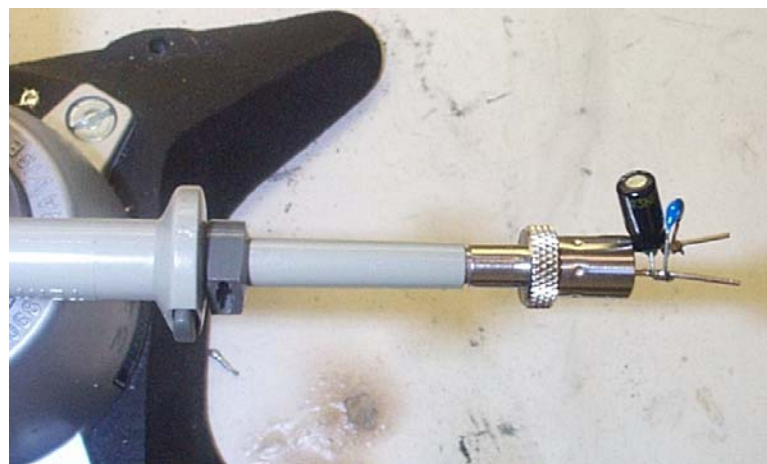
Figure 30 – Oscilloscope Probe with Probe Master 5125BA BNC Adapter (Modified with Wires as Probe Ground for Ripple measurement with two Parallel Decoupling Capacitors Added).
