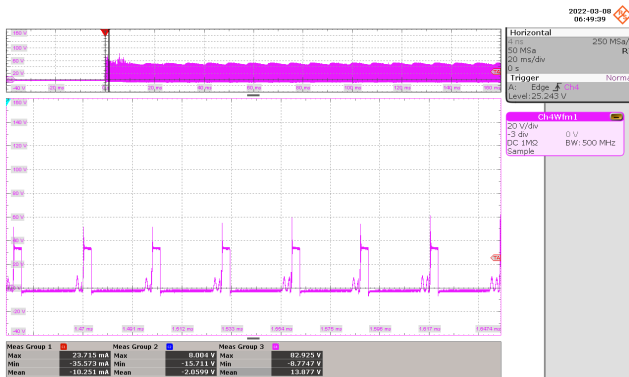
Figure 49 – 180 VAC 60 Hz, 20 V Full Load Start-up. CH1(Pink): V_{DS} , 20 V / div., 20 ms / div. V_{DS} = 82.925 V.
