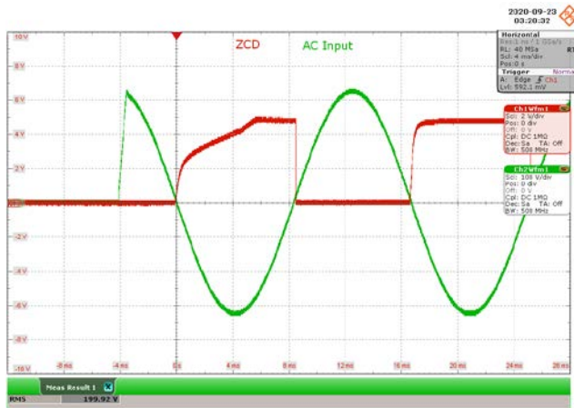
Figure 37 – 230 VAC 50 Hz, No Load. CH1: ZCD, 2 V / div., 4 ms / div. CH2: V IN , 100 V / div., 4 ms / div.
