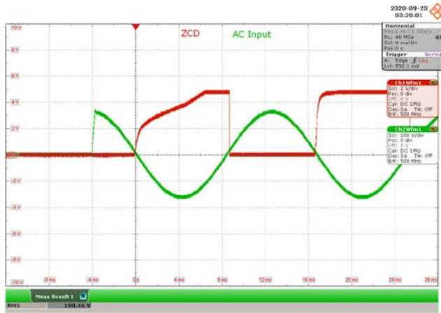
Figure 35 – 115 VAC 60 Hz, No Load. CH1: ZCD, 2 V / div., 4 ms / div. CH2: V IN , 100 V / div., 4 ms / div.
