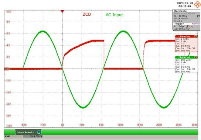
Figure 34 – 230 VAC 50 Hz, Full Load.
