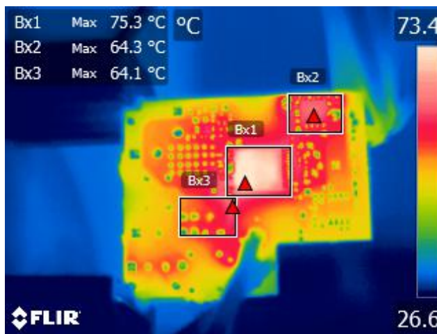
Figure 41 – Bottom Side Thermal Image. Bx1: InnoSwitch3-Pro = 75.3 °C. Bx2: SR FET = 64.3 °C. Bx3: Primary Snubber = 64.1 °C.
