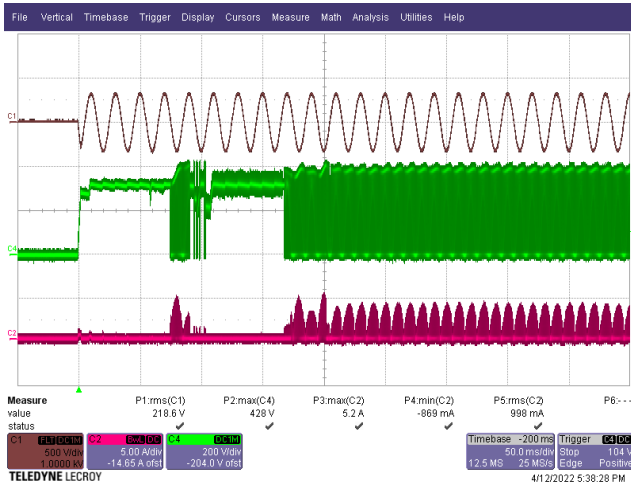
Figure 34 – PFC Inductor Current and HiperPFS-5. Drain Voltage at start-up 230 VAC. V_{DS\_PFS} = 428\text{ V} Maximum. I_{L\_PFC} = 5.2\text{ A} Maximum. CH1: V_{IN} , 500 V / div. CH2: I_{L\_PFC} , 5 A / div. CH4: V_{DS\_PFS} , 200 V / div. Time: 50 ms / div.
