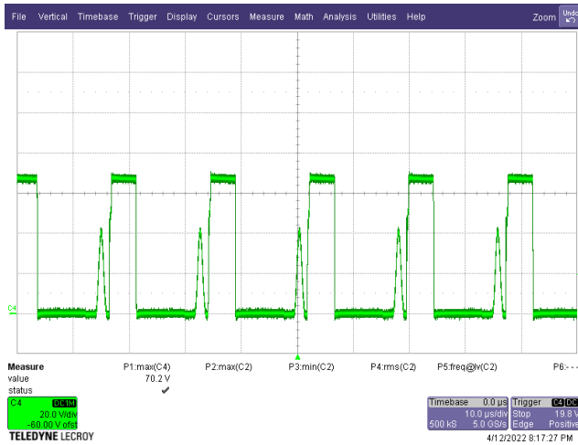
Figure 46 – SR FET Drain Voltage. 20 V, 9 A Load. V_{DS\_SRFET} = 70.2 Maximum. CH4: V_{DS\_SRFET} , 20 V / div. Time: 10 \mu s / div.
