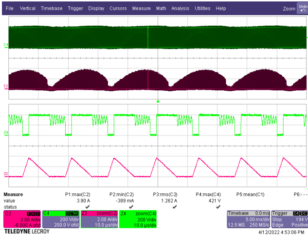
Figure 28 – PFC Inductor Current and HiperPFS-5. Drain Voltage 230 VAC. V_{DS\_PFS} = 421 V Maximum. I_{L\_PFC} = 3.9 A Maximum. CH4: V_{DS\_PFS} , 200 V / div. CH2: I_{L\_PFC} , 2 A / div. Time: 5 ms / div. (10 \mu s / div. Zoom).
