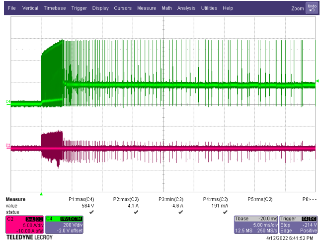
Figure 39 – Primary Drain Voltage and Current. 20 V, 0 A Load. V_{DS\_CPZ} = 584 V Maximum. CH4: V_{DS\_CPZ} , 200 V / div. CH2: I_{DS\_CPZ} , 5 A / div. Time: 5 ms / div.
